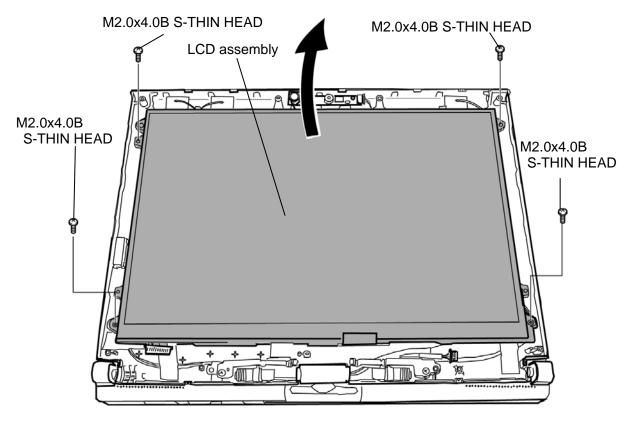
Figure 4-52 Removing the LCD assembly (1)
